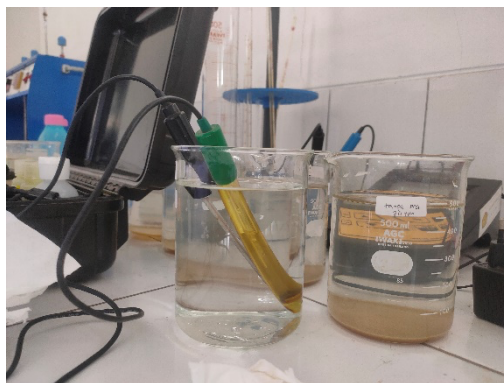
Figure 3 pH Testing Using a pH Meter
