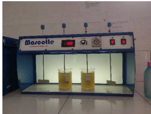
Figure 2 Coagulation and Flocculation Test Suit Method
